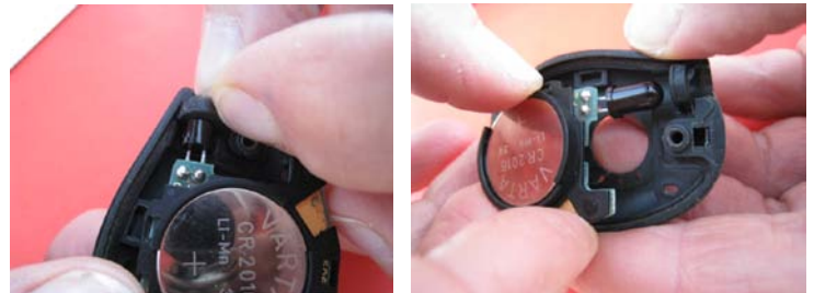
Now you can move electronic board and free up IR light from the rubber holding ring. To free up IR use your fingernail to push light gently thru the rubber hoop. At the same time you can gently pull board. You have to be careful not to lift up electronic board too high as you may break contacts on the light
