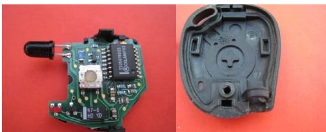
Once electronic board is separated from plastic part holding button you will be able to proceed to removal of an old rubber button.
