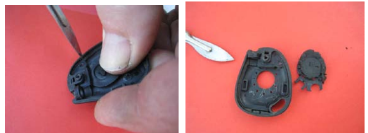
Using scalpel gently cut out worn button from the shell. Your clean shell is now ready for inserting a new Silicone Button
