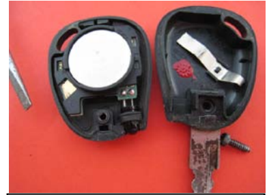
Once you open your remote you end up with button part holding battery and back part with key blade attached.
