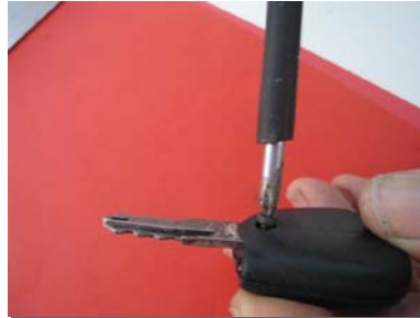
Use Phillips screwdriver to unscrew remote and than prise it open with flat screwdriver.
